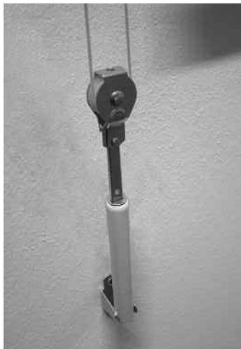
To fit the tension spring, put the control cord through the gap in the neck of the pulley. Position the tension spring at the maximum distance from the control mechanism, make sure it's at maximum tension and that the pulley is at the bottom of the loop. Fit the tension spring to the wall or window frame ensuring that cord remains under tension. The tension spring can be used on cords with a diameter of 1.7 - 2.2mm.
